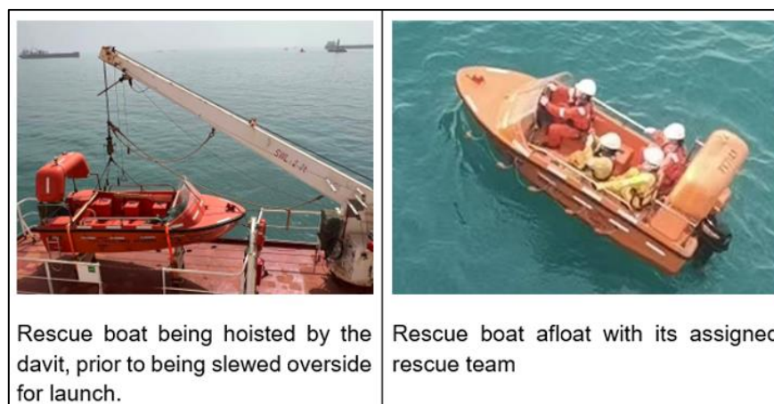
Figure 6: Photographs showing the rescue boat being hoisted and afloat in water after launching. (Source: The Company)
